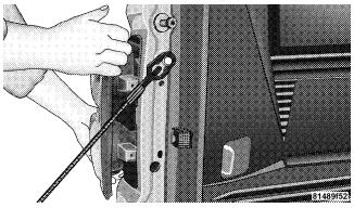
3. Rotate the bulb socket counterclockwise to remove it from the housing.
